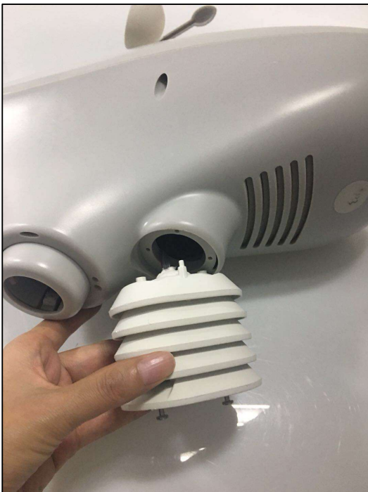
Figure 4: Installing a new sensor
