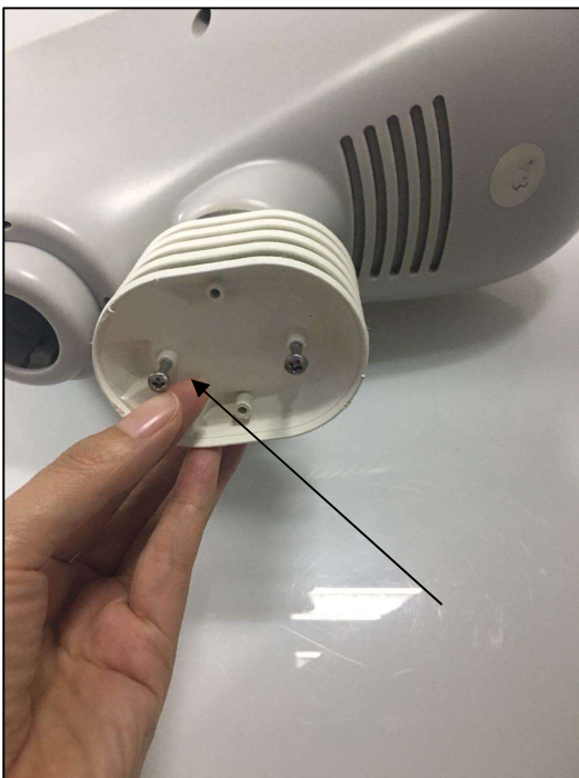
Figure 1: Removing the solar shield
