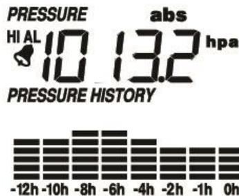
Press the **MENU** key five times to select the PRESSURE section, the PRESSURE section digits will start flashing. Press the **UP** or **DOWN** key to change between Relative and Absolute air pressure.
