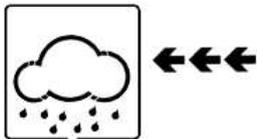
The storm threshold can be set to suit the user's requirements for storm forecasting - anywhere from 5-9hPa (default 4hPa). When there is a fall below the pressure threshold within any given 3 hour period the clouds with rain icon as well as the tendency arrows will flash for 3 hours indicating the storm warning feature has been activated.
